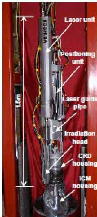
Fig. 7. PLP system for BWR bottom
